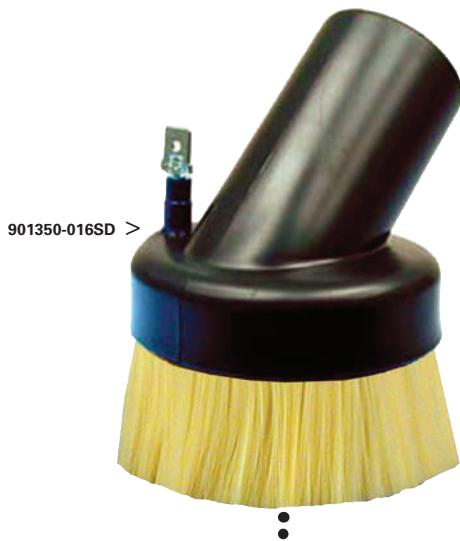
**Anti-Static Vacuum Brush:** Standard molded plastic vacuum head with grounding point, providing electrical continuity to the static dissipative filament. Use in static sensitive areas.
